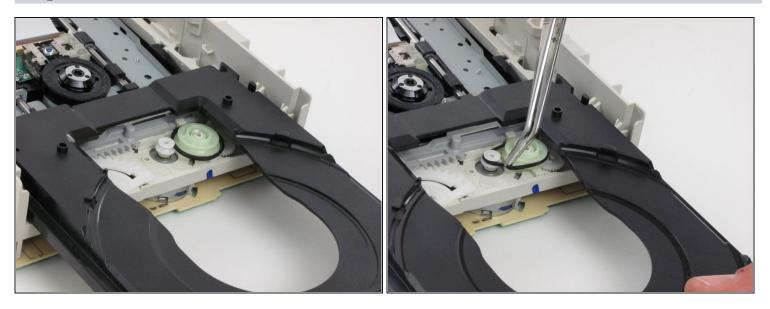
• Carefully replace with the new belt by wrapping it around the larger gear first, followed by the smaller gear.
