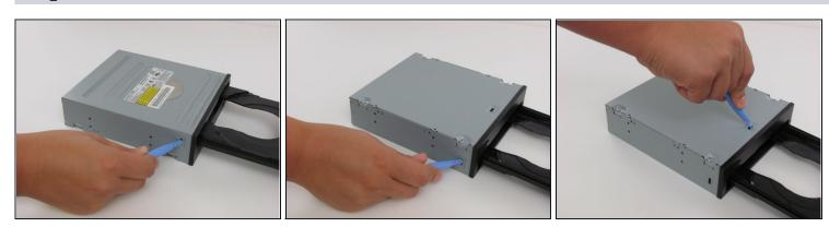
• Use an opening device to push in the black tabs on the left, right and bottom of the outer chassis to unhook the faceplate.
