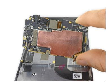
Lift the motherboard up and out of the device.
