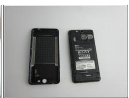
Remove the back case using plastic opening tool.
