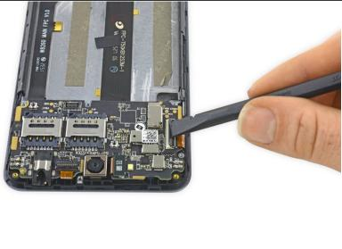
Use the flat end of a spudger to flip up the black retaining flap on the ZIF connector.
