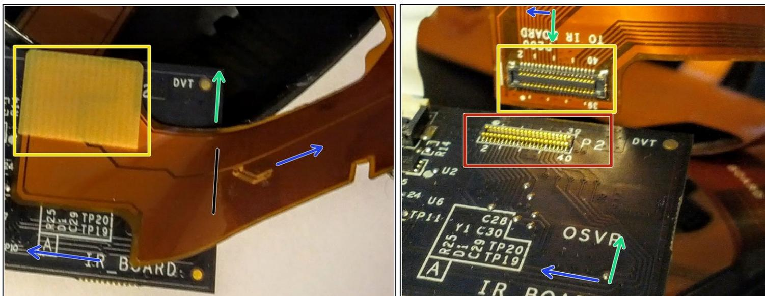
**i** This LED ribbon cable to IR board connection can be intimidating at first, because it feels "directly connected" to the board - but it's actually just a connector on the IR board face. The first two images are from a teardown of a modified 1.2 (you'll never see it like this in your own device) but they'll give a better idea of how it's connected.
