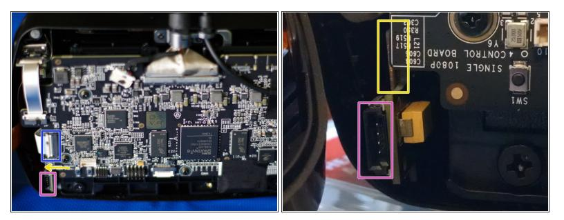
If you are following this guide to reprogram the IR board, and are able to use the "P5" programming connector - no more disassembly is required. The pink box indicates the location of P5 in an assembled HDK 1.x with the connector (1.4 units shipped with a P5-containing IR board).
