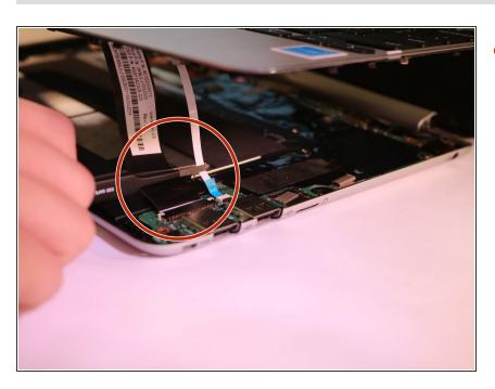
Disconnect the two cables from the motherboard with tweezers
