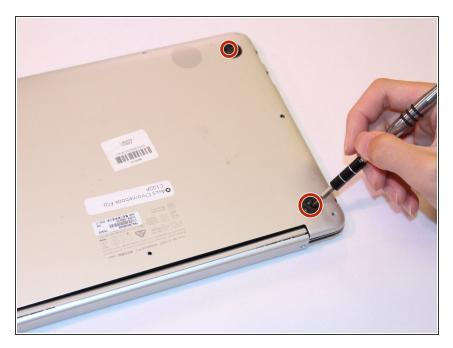
Unscrew the four screws under the feet using a screwdriver with a J100 tip.
