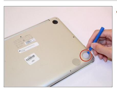
Use the plastic opening tool to remove the four bottom rubber feet.
