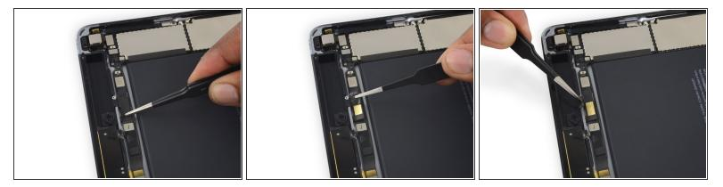
• Peel up the tape holding down the front facing camera's ribbon cable.
