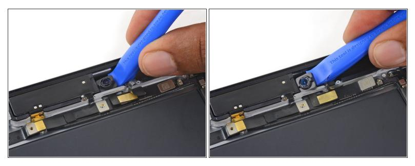
• Use a plastic opening tool to pry the front facing camera up from adhesive holding it in the iPad.
