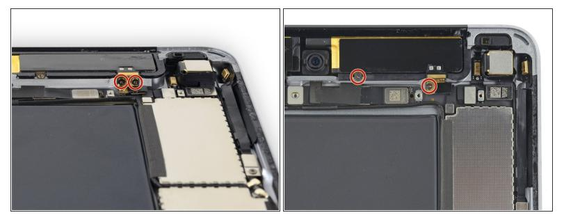
• Remove the four 1.3 mm Phillips screws securing the right antenna to the rear case.
