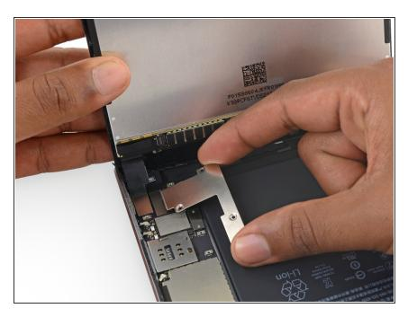
• Remove the battery/display cable bracket.
