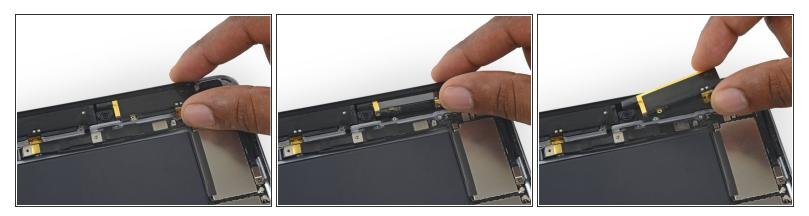
• Push the connector side of the antenna up and remove it from the iPad.
