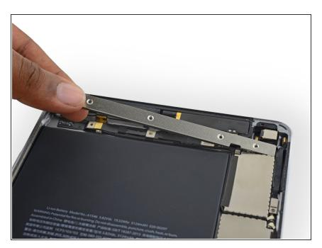
• Remove the upper component cable bracket.
