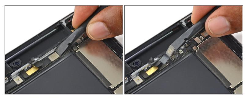
• Use a spudger to pry up the front facing camera's connector from its socket.
