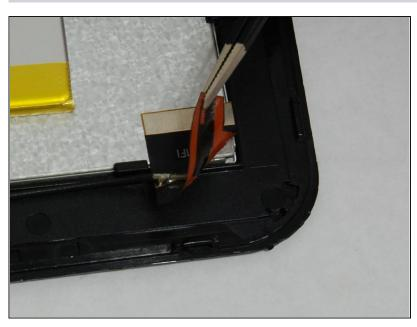
Next remove the WiFi module from the bottom of the device. This is simply pealed off.
