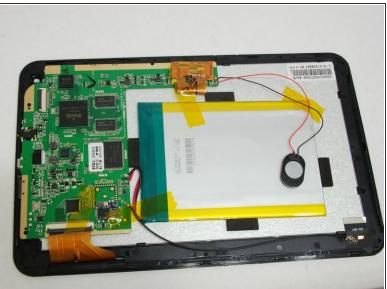
Using wide-tip tweezers, gently remove the three pieces of tape attached to battery
