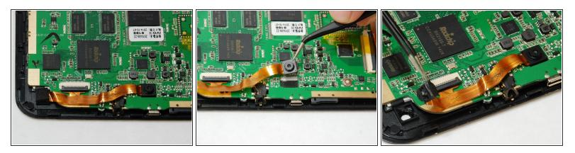
• Using hook tweezers, gently separate the glued cameras away from the circuit board.
