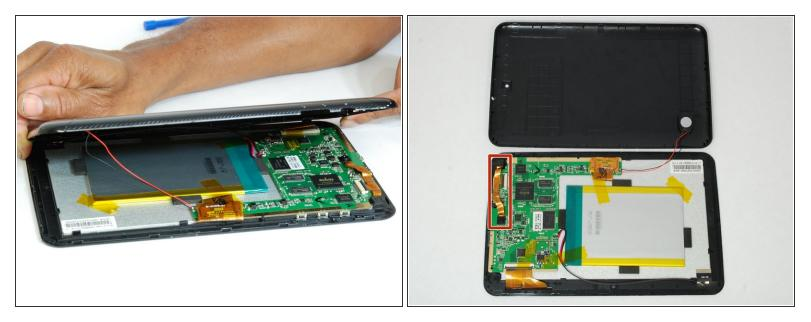
Once all connections have been loosened and using a soft surface, place the device onto its screen.
