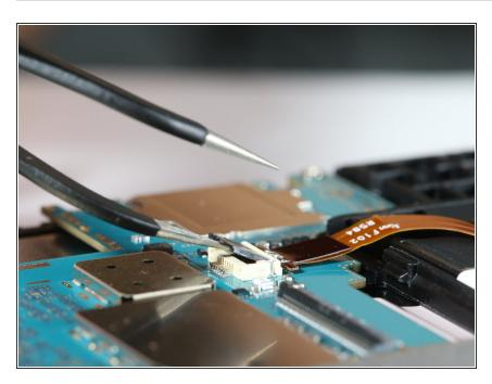
The second ribbon cable to remove is the wider, orange ribbon. The process is very similar to step 2.
