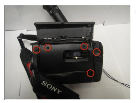
Use a Phillips #00 screwdriver to remove the five cassette side cover screws.
