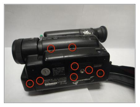
Use a Phillips #00 screwdriver to remove the eight screws located on the bottom of the camera.
