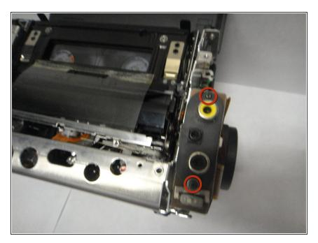
Use a Phillips #00 screwdriver to remove the two screws from the Input/Output.
