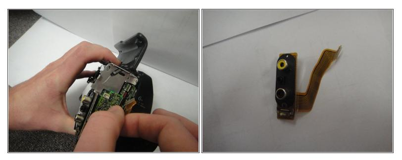
• Gently remove the Input/Output plug from the camera.
