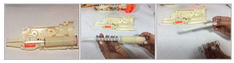
Remove the motor spring located inside the rotating barrel and replace.
