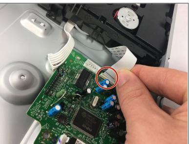
• Disconnect the white cables connected to the optical drive from the A/V board using your fingers.
