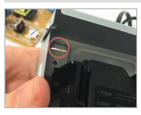
After removing the white wires connected to the A/V board, the optical drive should slide out of the slot. To reassemble your device, follow these instructions in reverse order.
