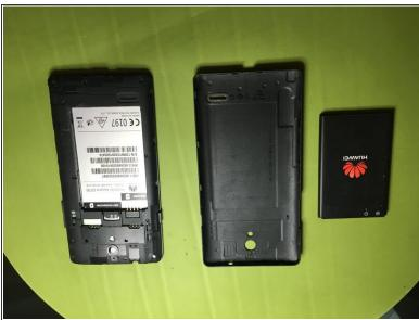
Remove the back cover and battery
