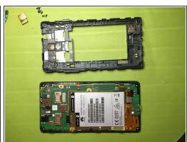
unhook Central frame using a thin tool behind joints along the entire perimeter of the phone
