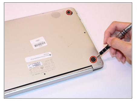
Unscrew the four screws under the feet using a screwdriver with a J100 tip.
