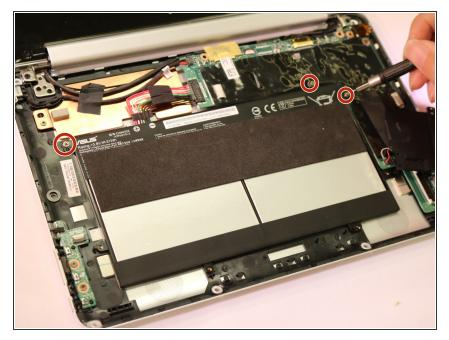
• Unscrew the three Battery Screws by using a screwdriver with a J00 tip.
