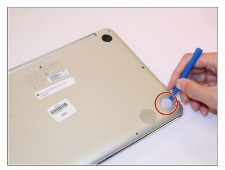
• Use the plastic opening tool to remove the four bottom rubber feet.
