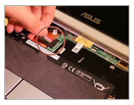
Lift the battery cable out of Mother Board
