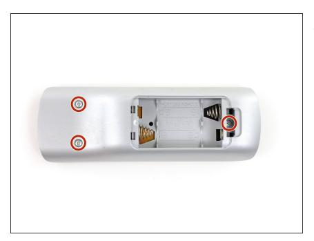
Remove the three 9mm Phillips #00 screws located on the backside of the remote.
