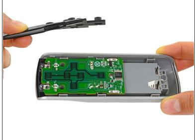
Lift the button pad up and out of the remote.
