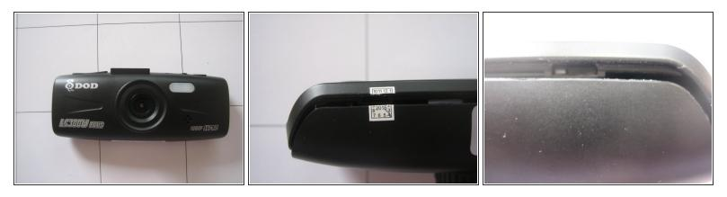
Using an opening tool, pry open the seam on the bottom of the dash cam to separate the two parts of the device.
