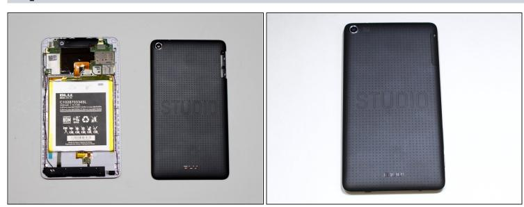
② Once the back has been removed, you can snap the new one into place by pressing firmly around the edges with your fingers.
