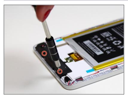
Remove two 3mm screws from the bottom black panel.
