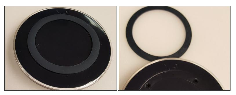
Remove the padding by using a flat tool to remove adhesive and pry padding off of device. Be careful not to rip or tear.
