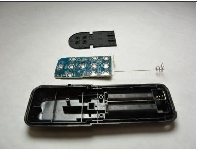
• Use the opening tool to lift the back of the motherboard. Slowly lift the motherboard while keeping the wires straight.
