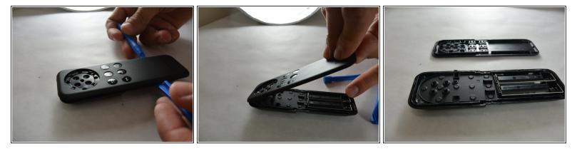
Use two plastic opening tools to pry along the seam of the remote and separate the face plate.
