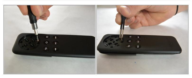
Remove the 6mm triangle head screw on the front of the remote.
