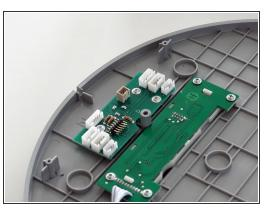
Remove the dock sensor from the circuit board. Grip the small white tab on the side and pull up.
