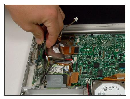
Lift the DC & sound card out of lower case, but don't remove it entirely as there are still cables connected.
