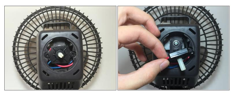
• The motor switch is also free and can be removed by hand to reveal a screw holding the housing assembly in place.
