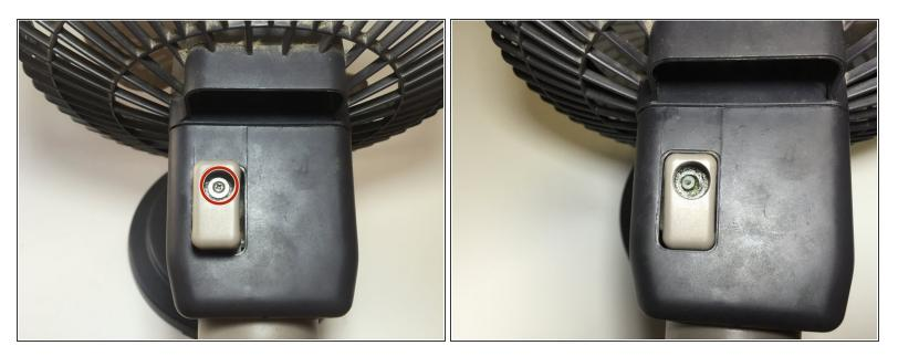
On the top of the fan, there is a screw fastening the oscillation button to the gear train within the housing. Remove this screw with the Phillips #0 Screwdriver.
