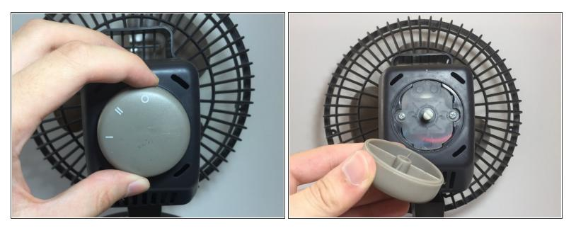
• The on/off and fan speed nob can be removed by simply pulling it away from the main housing.
