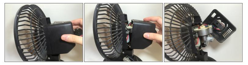
• The housing assembly can now be pulled off and pushed to the side to reveal the fan motor and gear train.
