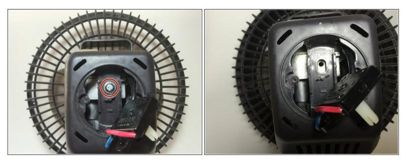
• Remove the screw that holds the housing assembly in place by using a Phillips #2 Screwdriver.
