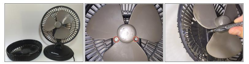
• Using a 7 mm socket and wrench, remove the 2 nuts that are behind the fan blades.
