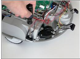
There is one screw holding each edge sensor in place. Remove all four screws and keep them aside for reassembly.
