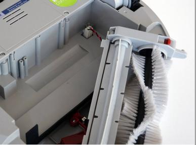
Pull the brush compartment up until it is freed from the red fastener. Then, detach the brush compartment and set it aside.
