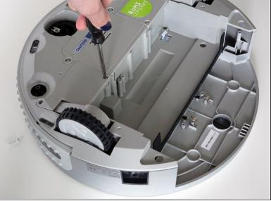
Remove the two screws holding the wheel you'd like to replace. In this case, bObi Pet's right wheel
