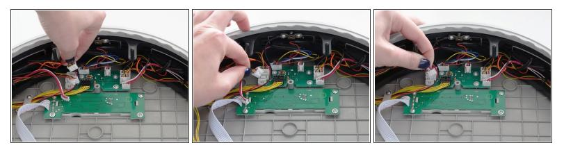
(i) The rows on each side of the cover circuit board follow the same pattern for installation.
