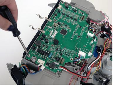
Next, remove the 4 screws holding the mainboard down. Keep these closeby for the next step.
