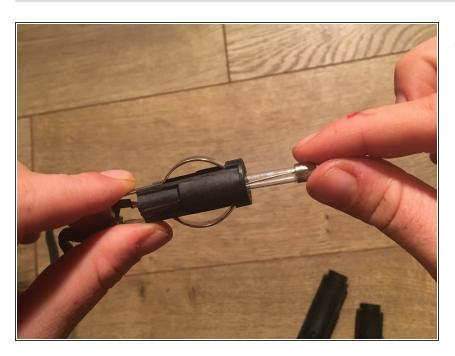
Remove the 15 amp fuse and replace.
