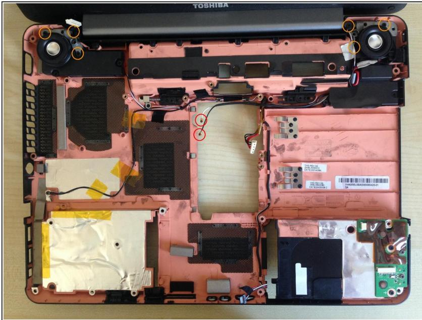
**⚠** Before attempting to remove the screen or any other components left in the shell, make a careful note of how each cable is routed. Take detailed photos if your laptop is not identical to this one.
