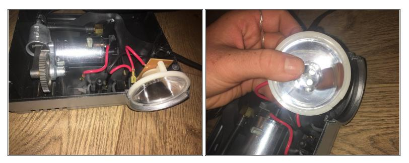
• Remove the **light fixture** from the slot in the front.
