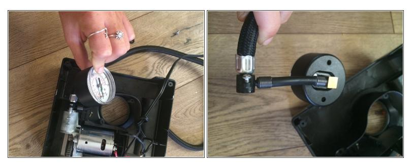
• Remove the pressure gauge.
