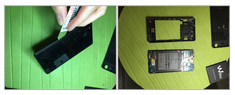
using a thin tool separate the middle frame from the body display
