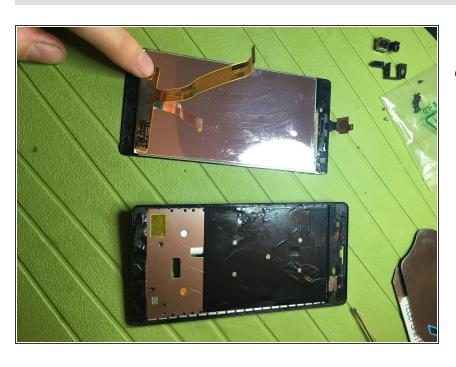
With heat and and an small ESD tweezers lift the glass from the frame and extract touch screen and display from the phone body To assemble the device, follow these instructions in reverse order.
