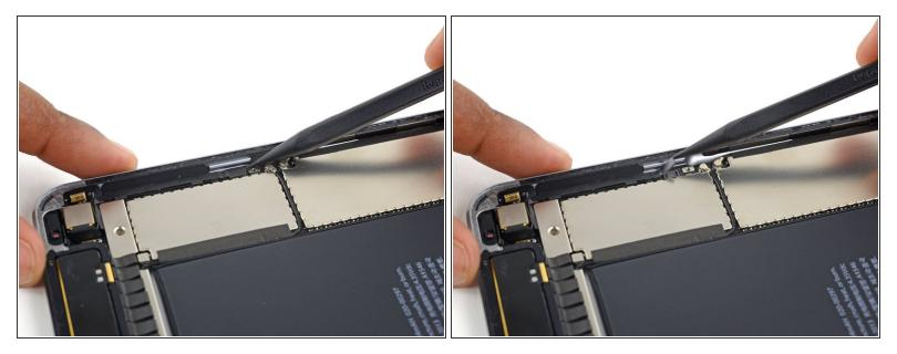
• Lift the ribbon cable connector up off its socket on the logic board.
