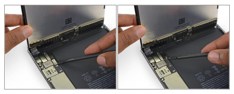
Mhen disconnecting any press connectors from the logic board, be sure to lift the connector straight up to avoid ripping the socket off the board.
