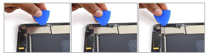
Slide an opening pick underneath the volume control buttons' ribbon cable to peel it away from the adhesive below.
