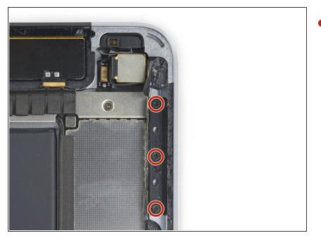
Remove the three 1.8 mm Phillips screws securing the volume control assembly to the rear case.
