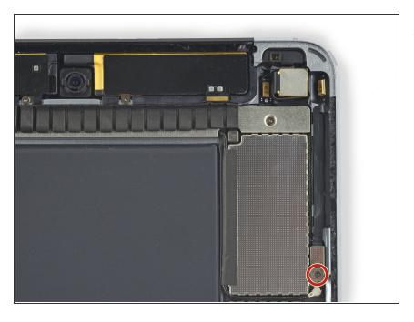
Remove the single 1.2 mm Phillips screw securing the volume control cable bracket.
