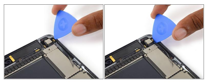
• Use a plastic opening tool to pry the microphone off the rear case.
