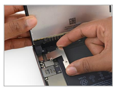
• Remove the battery/display cable bracket.
