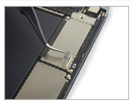
• Remove the volume control cable bracket.
