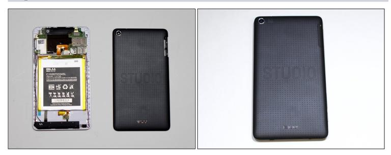
Once the back has been removed, you can snap the new one into place by pressing firmly around the edges with your fingers.
