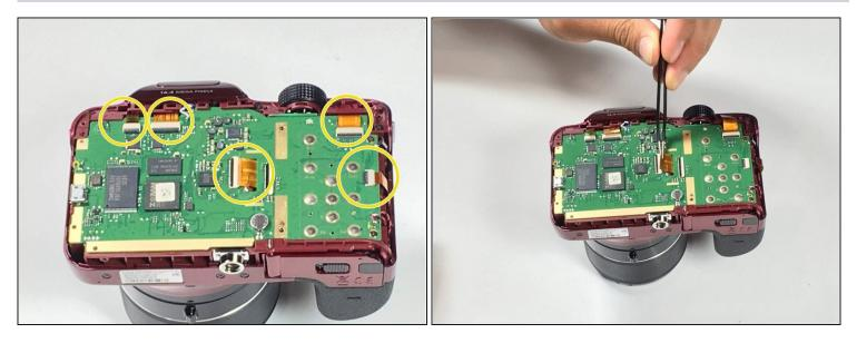
• Use the tip of a spudger or your fingernail to flip up the small retaining flaps on the five ZIF connectors on the motherboard.
