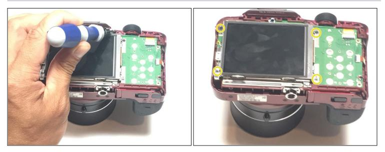
• Remove four 1.2 mm Phillips #1 screws connected to the LCD screen.
