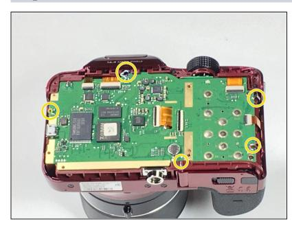
• <u>Desolder</u> five wires connected to the camera motherboard.
