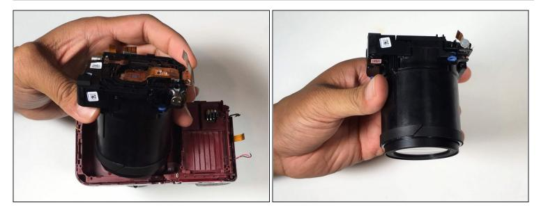
• Pull the lens assembly from main body of the camera, using a spudger to pry if necessary.
