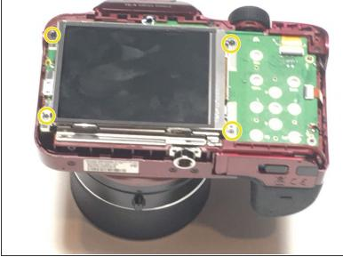
Remove four 1.2 mm Phillips #1 screws connected to the LCD screen.
