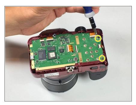
Remove two 1.2 Phillips #00 screws connected to the motherboard.
