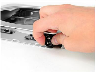
Rotate the AC-In connector 90 degrees counter-clockwise.
