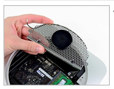
Remove the antenna plate from the mini.
