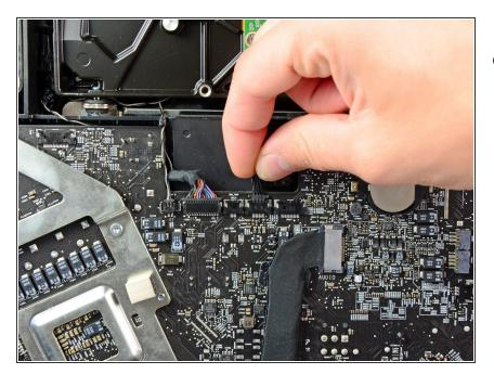
Pull the hard drive fan connector toward the top edge of the iMac to disconnect it from its socket on the logic board.
