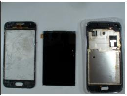
If you want to change only the glass, disconnect the touch screen flex cable and gently separate the glass from the LCD.
