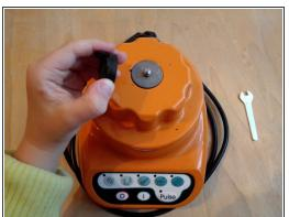
Loosen the defective coupling with water pump tongs and original open-ended spanner. Hold the axis with an open-ended spanner and unscrew the coupling. Remove coupling.
