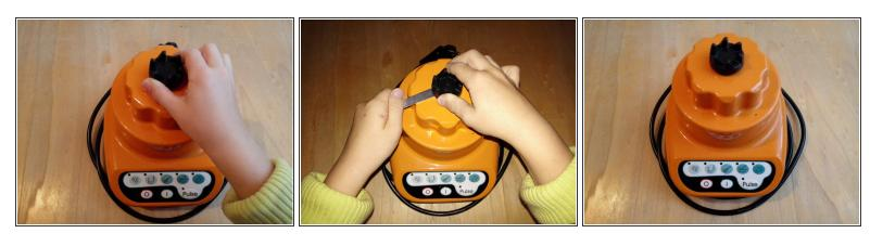
Insert the new coupling and screw it on slightly. Screw the new coupling by hand with a spanner.
