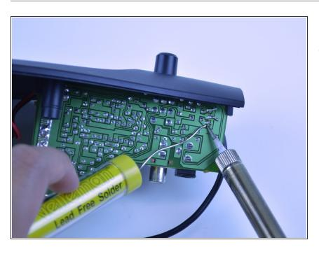
Use the soldering iron to flow solder between each wire and its solder pad.
