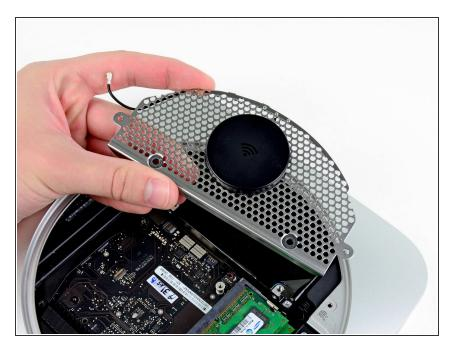
Remove the antenna plate from the mini.
