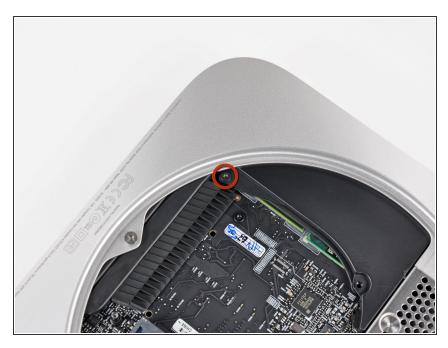
Remove the single 3.5 mm T6 Torx screw securing the cowling to the heat sink.
