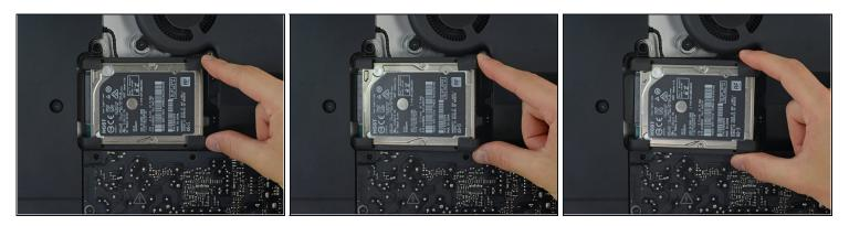
• Lift the hard drive from the edge nearest the logic board and pull it slightly out of its recess.
