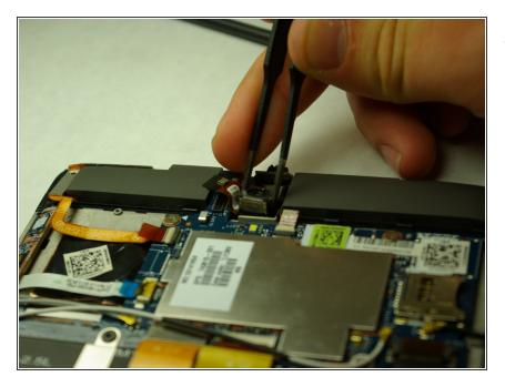
Use the tweezers to pry the camera assembly away from the motherboard.
