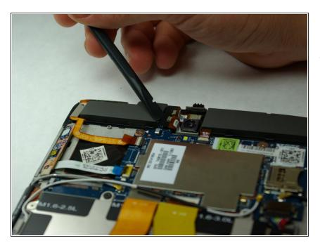
Use the Spudger to disconnect the ribbon cable to the rear facing camera.
