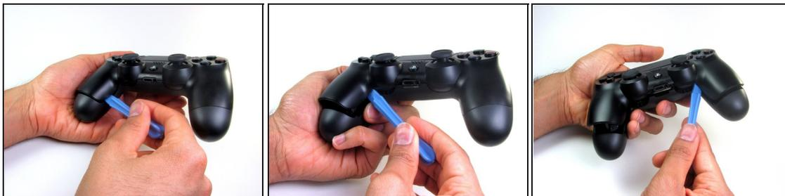
**i** Four fragile plastic clips hold the casing together. You can see their locations more clearly in [this guide](#).
