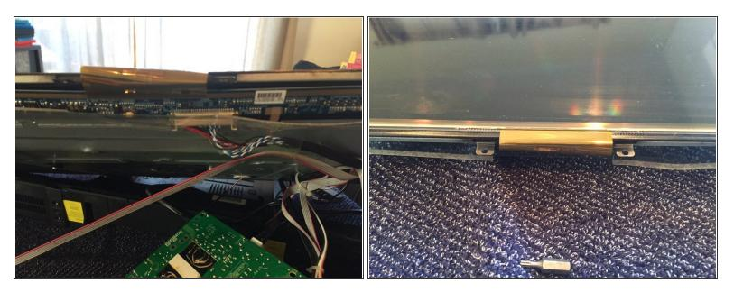
Now that the screen has been removed, take the new screen and attach its circuitry in the same place as the previous screen. After that, connect the cable from the rest of the TV to the screen's port and it should be good to go!
