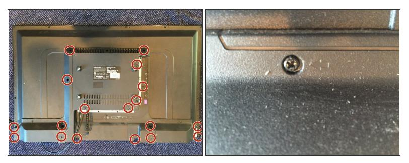
To begin removing the back plate, find and remove all 18 screws indicated with the Phillips screwdriver.
