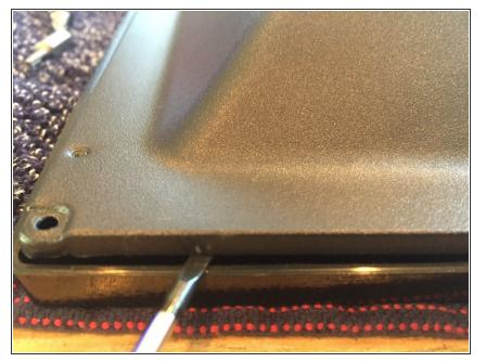
Once the screws are all removed, slide the flat-head screwdriver into the small gap between the front and back plates. Use the screwdriver to pry the plates apart and lift the back plate up.
