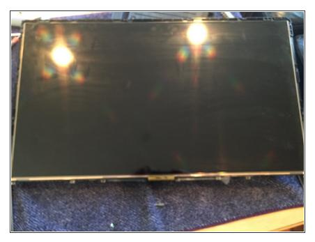
• Completely separate the back from the front and flip the back section over so that the screen is now on top.
