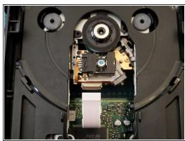
Gently press back on the ribbon retention tab and pull back on the ribbon cable
