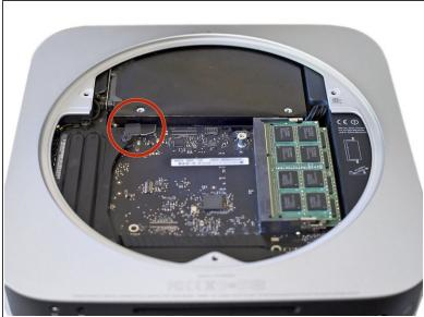
Use the flat end of a spudger to pry the hard drive connector up from its socket on the logic board.
