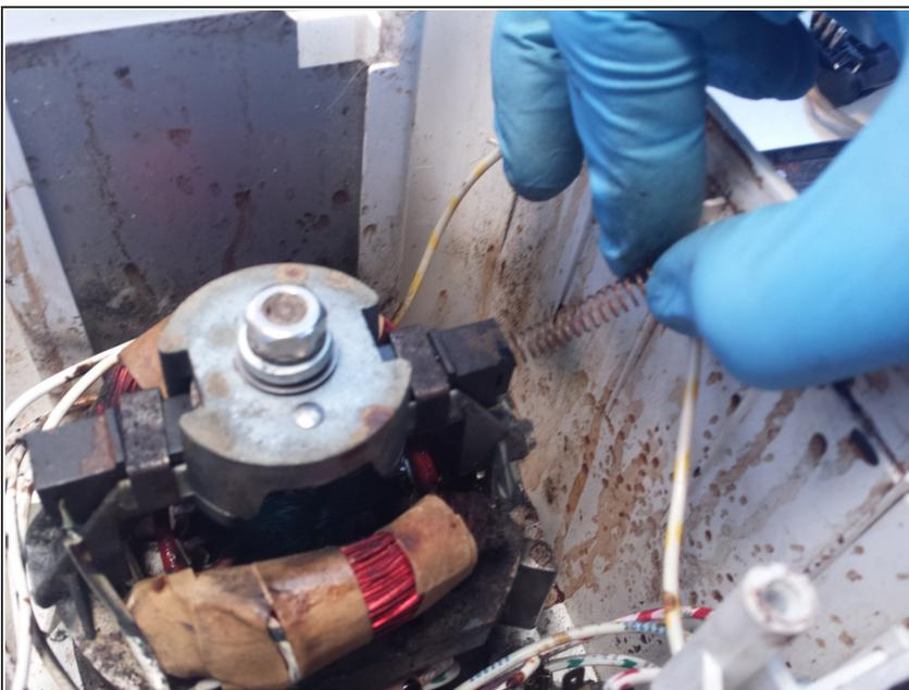
⚠ After you remove the first connection, this motor brush will begin to come out but do not remove it completely.
