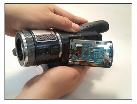
Take off the top and bottom screws on the LCD shell
