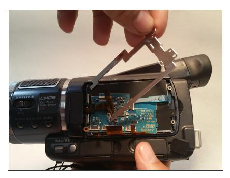
Remove screws from the metal shield that is situated on the microchip
