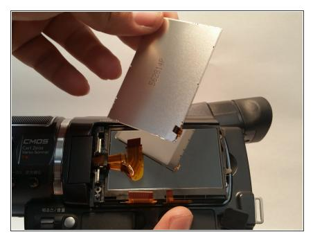
• Remove the LCD in the shell
