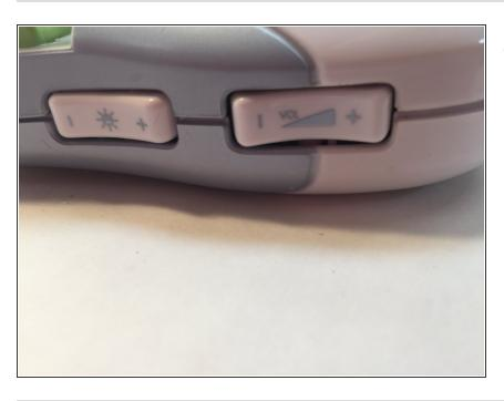
Place the new button on top of the unit and place the top over as shown.
