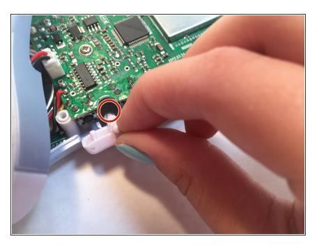
Remove broken side button used for volume.
