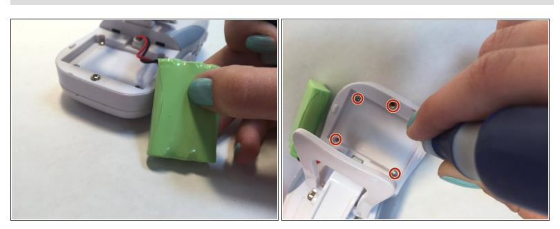
Remove four 3mm screws below the battery.
